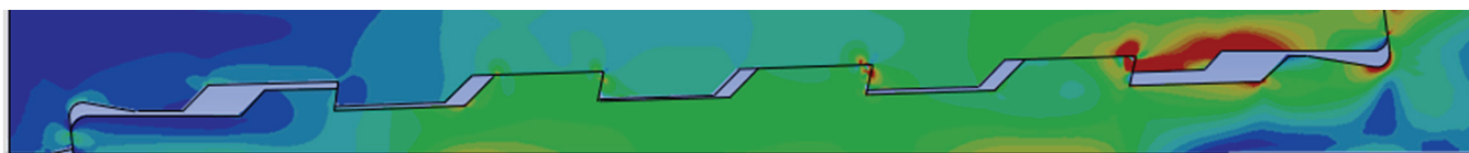
Figure 2 - A typical representation of how preload stress sits in a single start thread using heat mapping. Stresses within the connection typically concentrate near the final full wrap of the pin thread (shown on the right side of the model).
